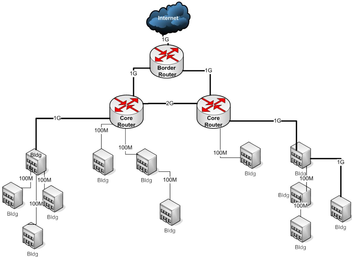
Figure 1. Illustration of current network topologies on the CSU campus, with multiple buildings often behind a single connection to the campus backbone network.
