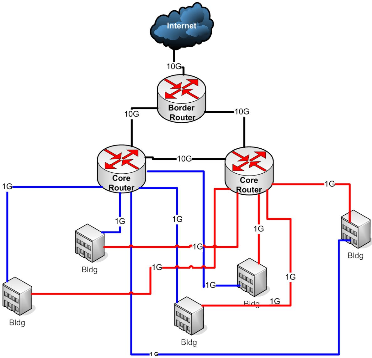
Figure 2. Illustrates a topology where buildings are connected via primary and backup gigabit Ethernet connections.
